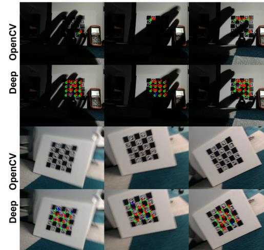
Figure 7: Detector performance comparison under extreme shadows (top) and motion (bottom).
