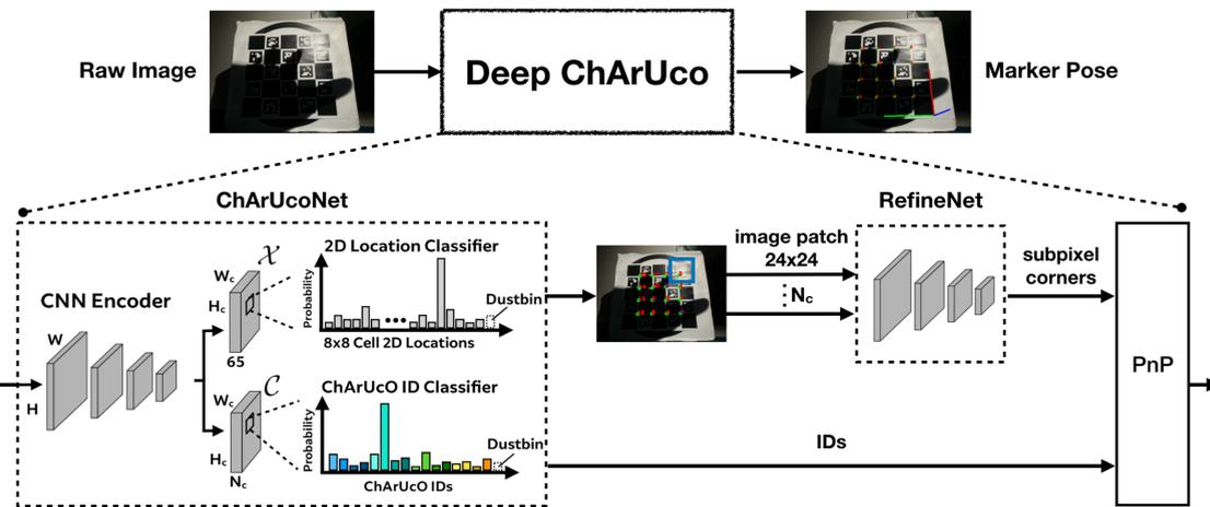
Figure 1: Two-Headed ChArUcoNet and RefineNet. Both **ChArUcoNet** and **RefineNet** are SuperPoint-like [1] networks using VGG-based backbone:
